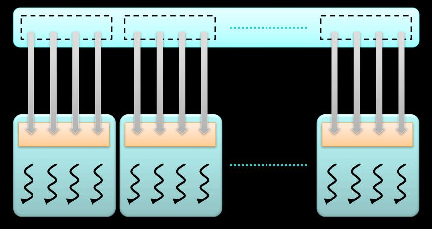
Load the subset from global memory to shared memory, using multiple threads to exploit memorylevel parallelism
